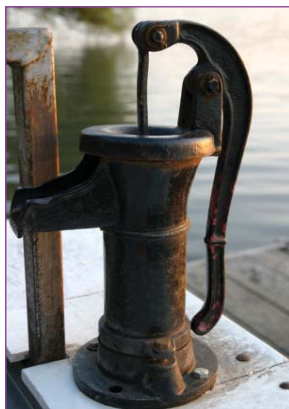
The handle of this old-fashioned water pump is an example of a first-class lever.
