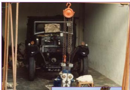
A mechanic may use pulleys to remove an old engine from a car.
