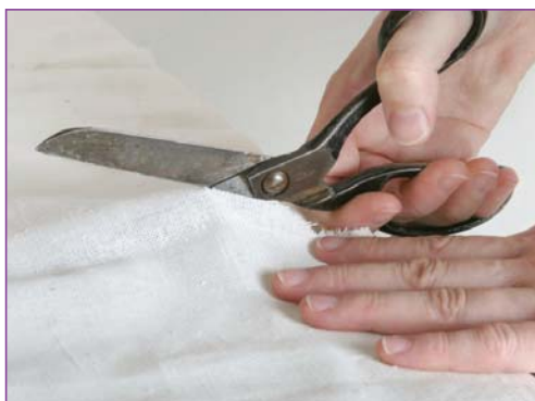
Scissors are made up of two first-class levers joined together at the fulcrum. The cutting edges are wedges.
