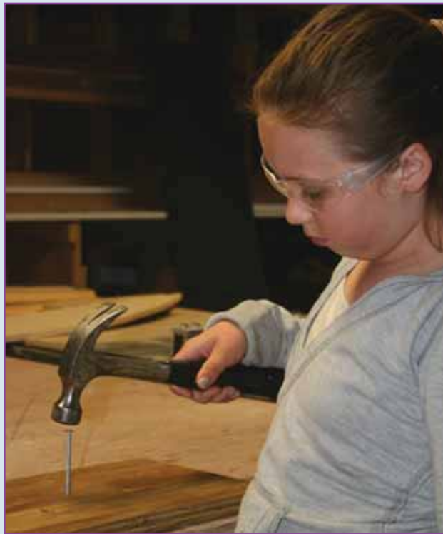
To move the nail into the wood a hammer applies a large, unbalanced force on the top of a nail.
