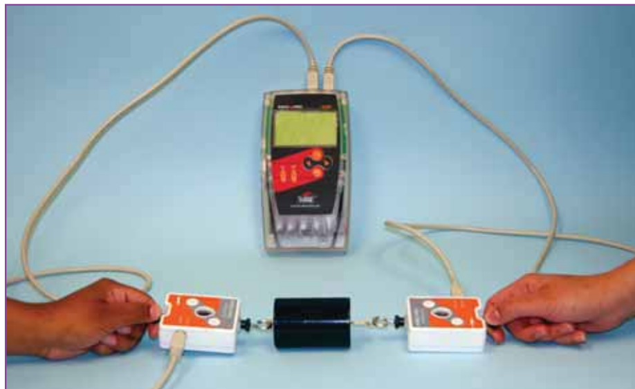
A force probe is an instrument used to measure the amount of force applied to an object.
