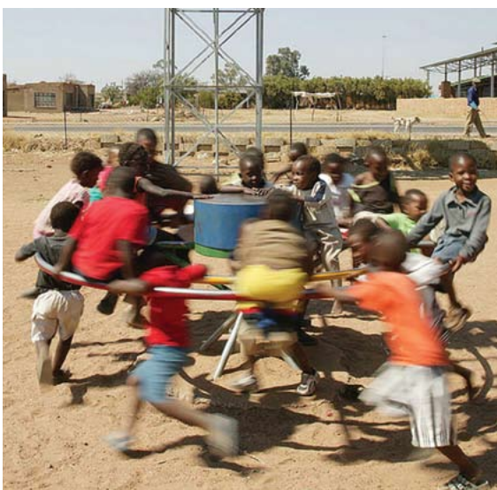
Children playing on this merry-go-round provide the energy to power a water pump.
